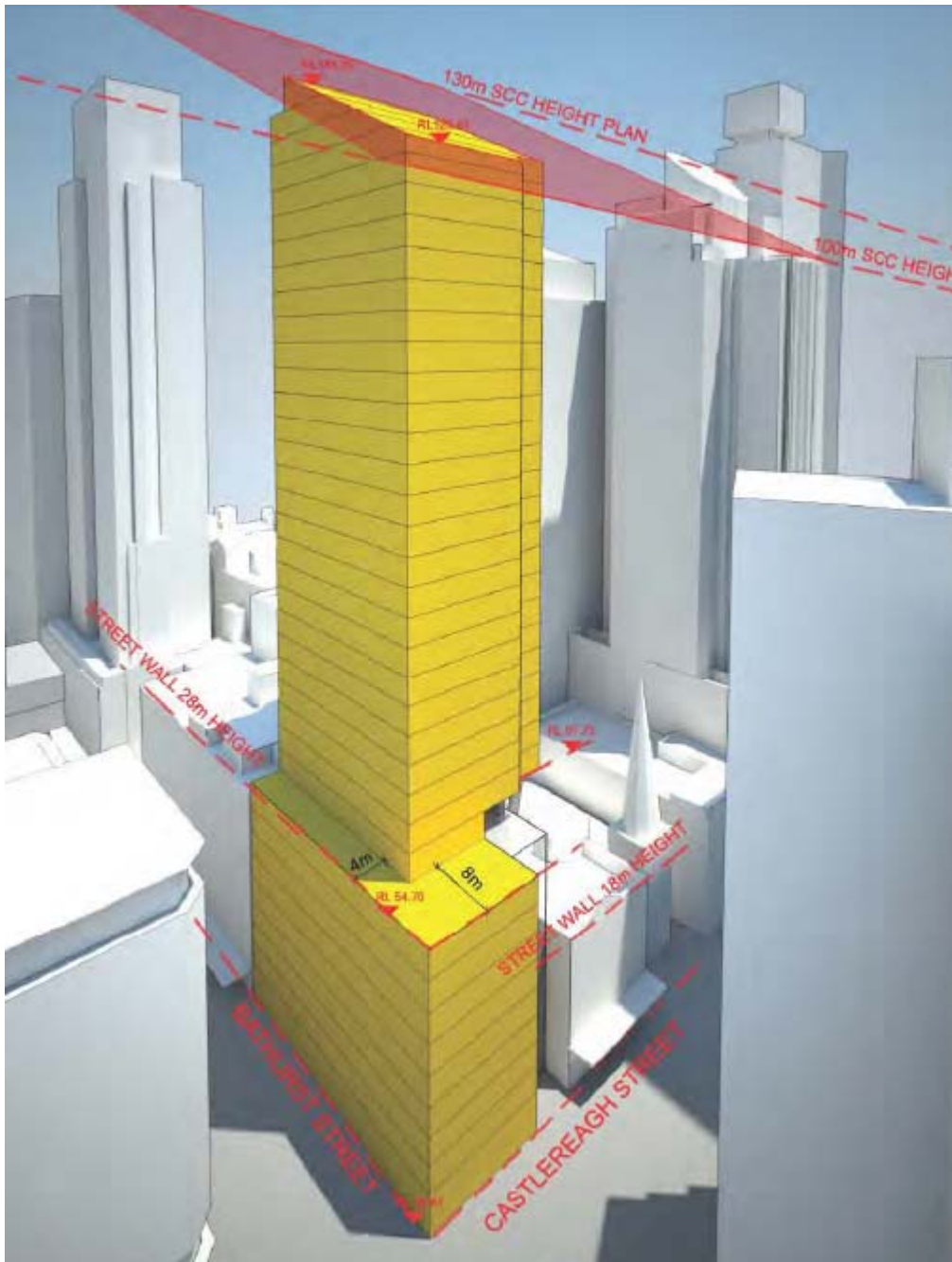
Figure 4: Proposed building envelope, viewed from opposite corner of Bathurst Street/Castlereagh Street intersection.
